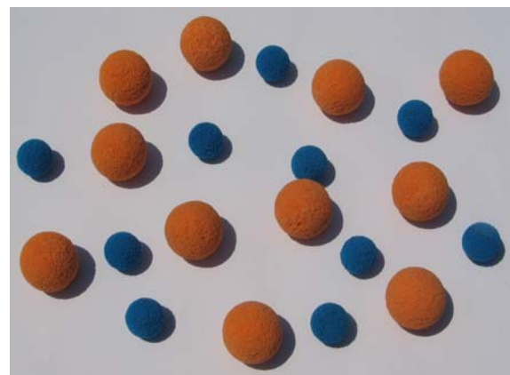
The two sizes of Taprogge balls used at Eraring Power Station
